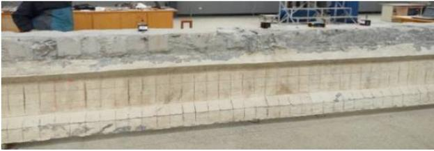
Fig. 2. Grid Lines for Observation of Main Beam Cracks
