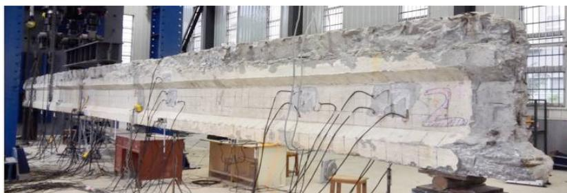
Fig. 12. Strain Measuring Point Arrangement of Undamaged Beam
