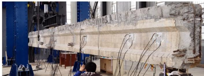
Fig. 11. Strain Measuring Point Arrangement of Damaged Beam
