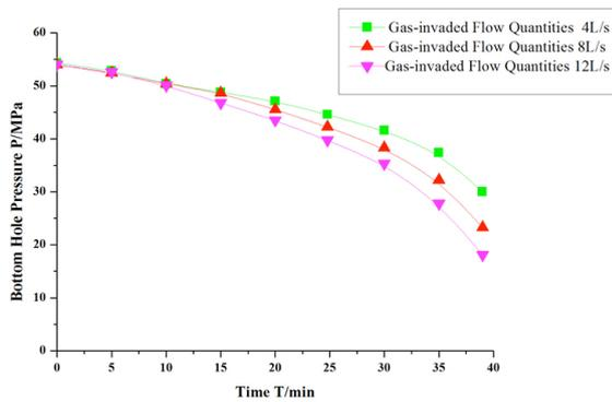
Fig. 10. Comparison Curves of Bottom Hole Pressure with Time under Different gas-invaded Flow Quantities
