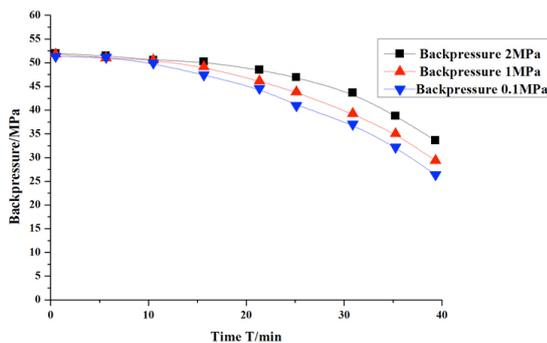
Fig. 11. Comparison Curves of Changes of the Bottom Hole Pressure with Time under Different Backpressures
