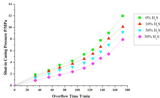
Fig. 9. Change Curves of Shut-in Casing Pressure with Overflow Time
