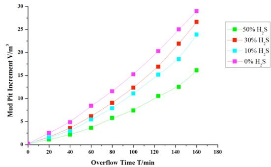
Fig. 8. Change Curves of mud pit Increment with Overflow Time
