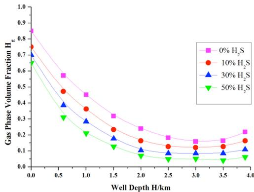
Fig. 7. Gas Phase Volume Fraction in the Wellbore when the Gas Rises to Wellhead
