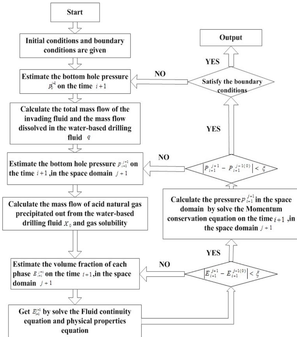
Fig. 1. Solving Process of a Wellbore Flow Model
