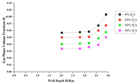
Fig. 6. Gas Phase Volume Fractions in the wellbore when the Gas Rises to Its Middle Position
