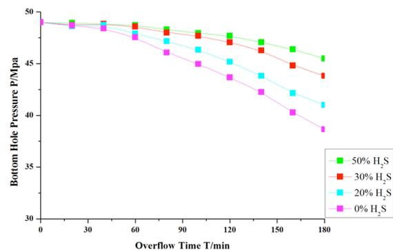
Fig. 5. Change Curves of Bottom Hole Pressure with Overflow Time
