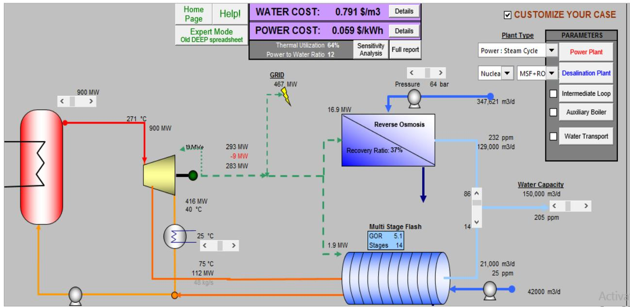
**Fig. 2.** Simulated case using DEEP
