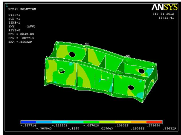
Fig. 6. Stresses in X directions (Sx) of composite foundation
