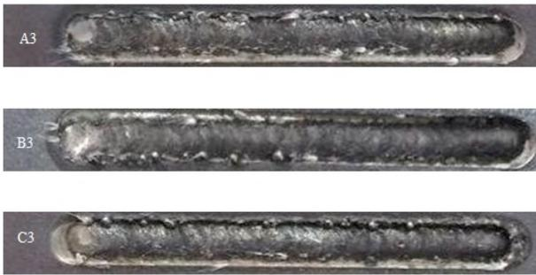
Fig. 4. Macro morphology of the cladding layer at different scanning speeds
