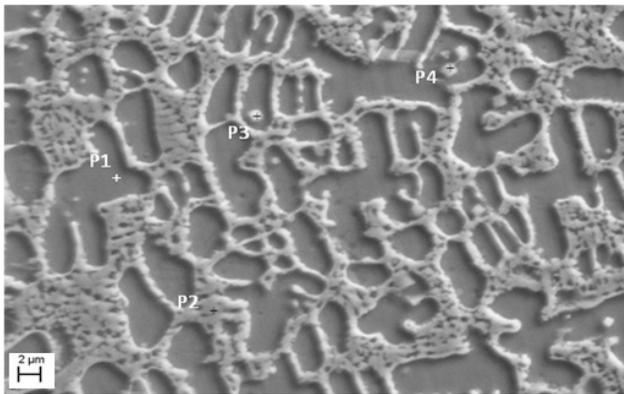
**Fig. 8.** Microstructure of the Ni60A+24%(SiC+Ti) composite coating
