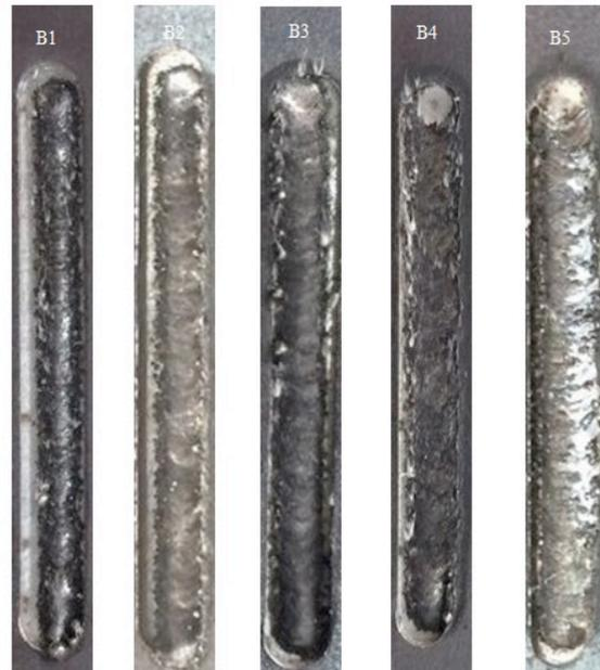
**Fig. 3.** Macro morphology of the cladding layer at different laser power values
