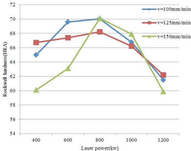
Fig. 5. Effect of laser power on the hardness of the cladding layer
