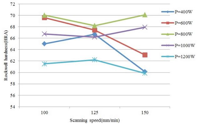
Fig. 6. Effect of scanning speed on the hardness of the cladding layer
