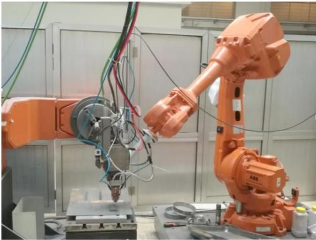
**Fig. 1.** Laser cladding system
