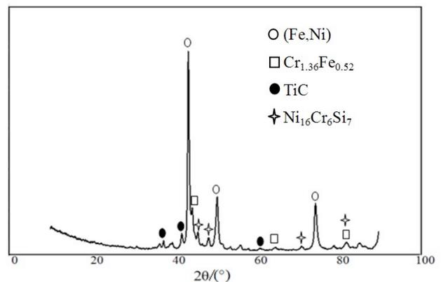
Fig. 7. XRD spectrum of the Ni60A+24%(SiC+Ti) composite coating
