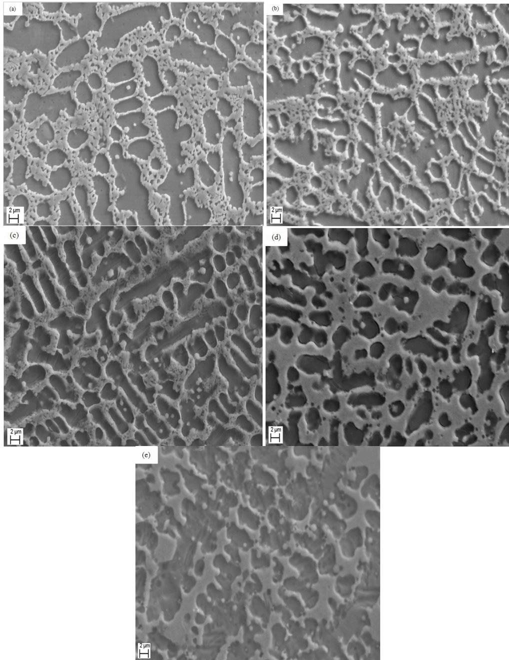
(a) Ni60A+12%(SiC+Ti). (b) Ni60A+24%(SiC+Ti).
