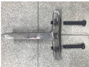
(c) Failure Mode 3: Deformation of the specimens and the finite element model
