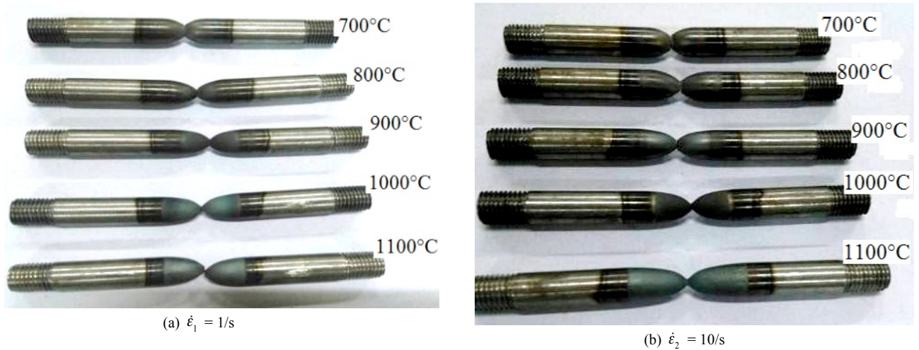
Fig. 7. Specimens at different temperatures and strain rates after fracture
