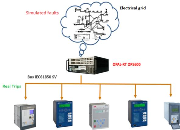
Fig. 8. Integration and conjunction operation through OPAL-RT
