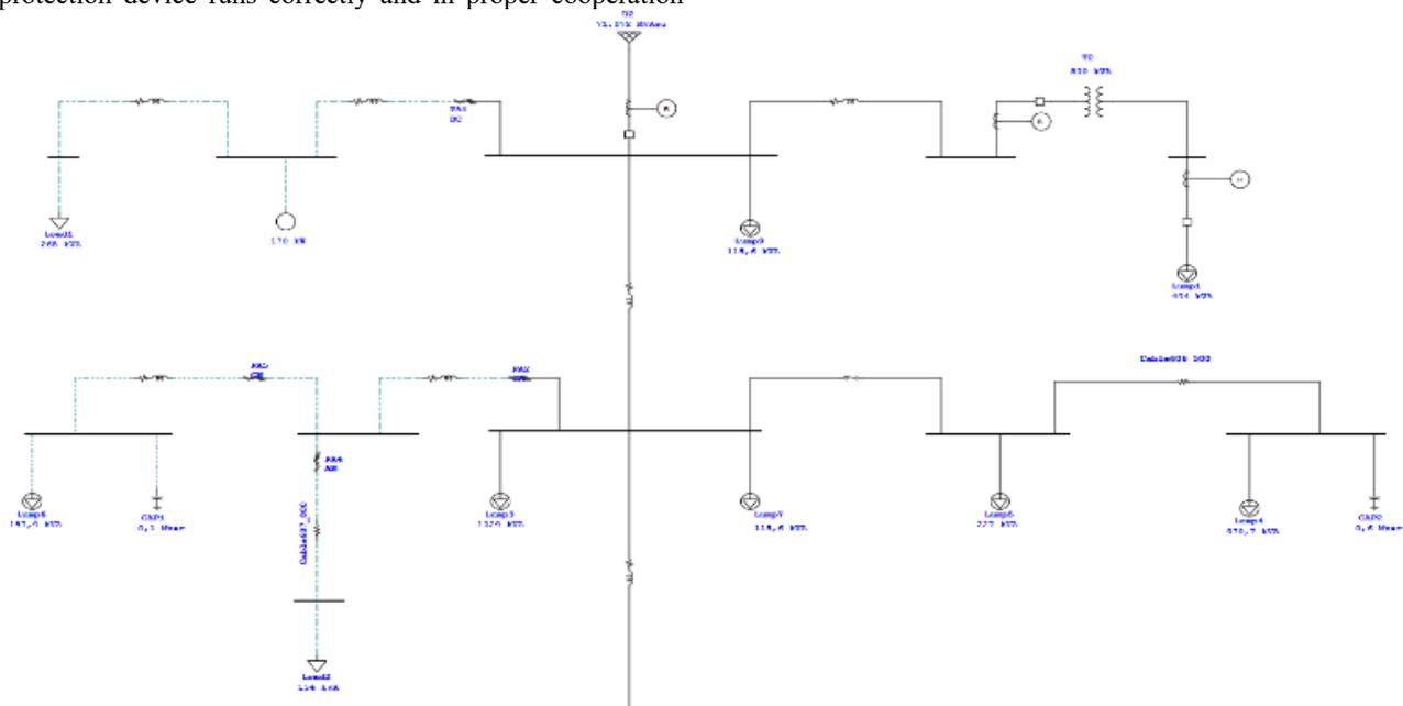
Fig. 10. ETAP – IEEE 13-node test feeder
