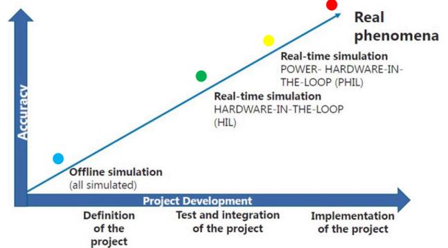
Fig. 7 shows how the main objective of this technology is to approach the real phenomenon and with tools such as HIL and PHIL, this is possible.
