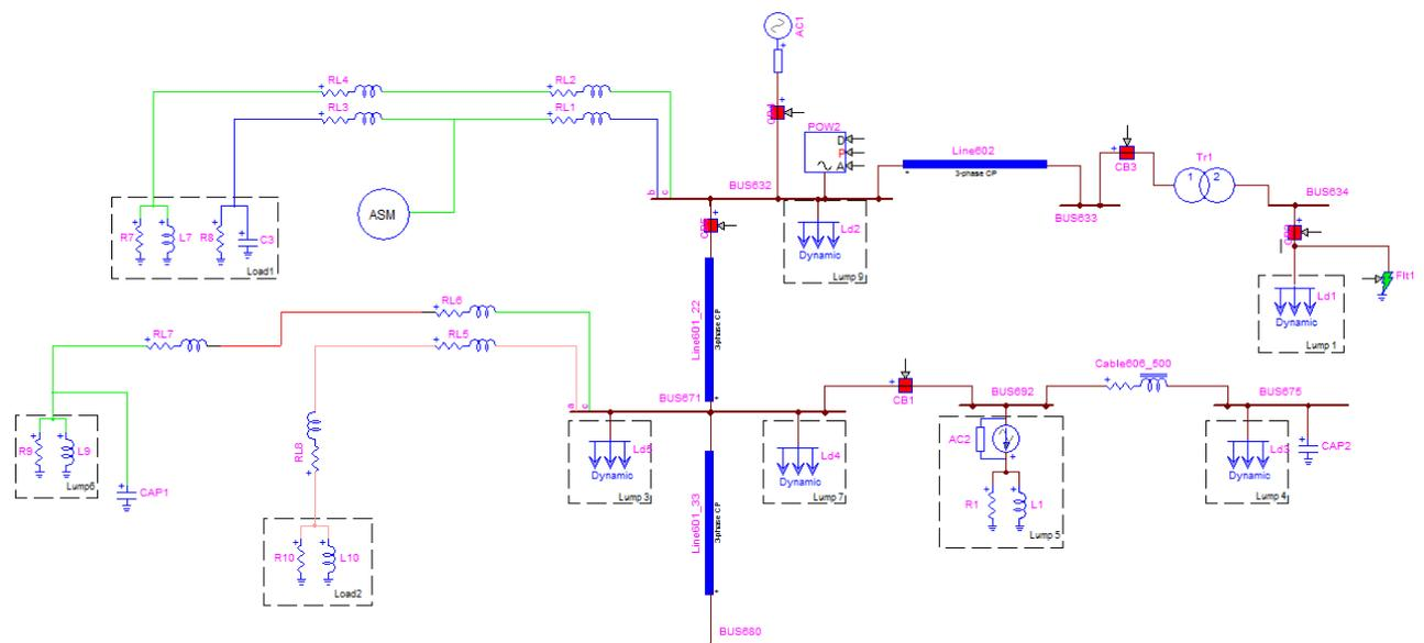
Fig. 13. IEEE 13-node test feeder implemented in HYPERSIM
