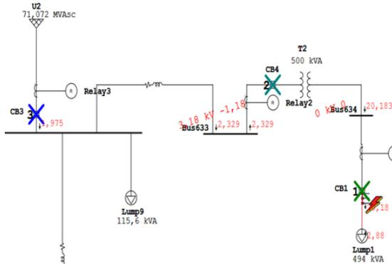
Fig. 11. Sequence of operation of protection devices
