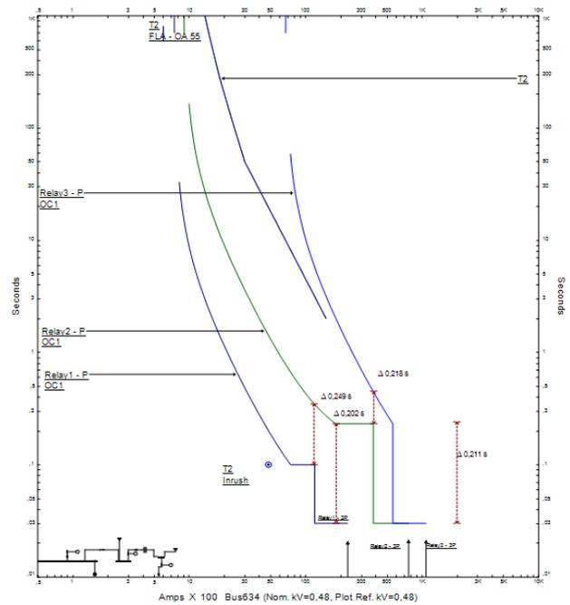
Fig. 12. Selectivity diagram of overcurrent protections
