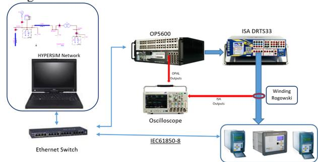
Fig. 9. PHIL model for integration of protection devices and IEC61850-8
