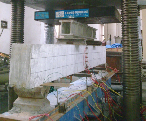
Fig. 2. Practical loading for specimens.
