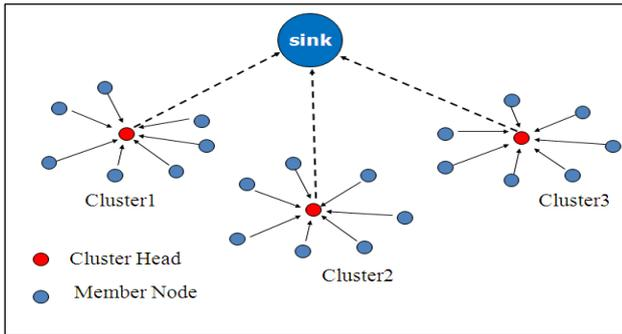
Fig. 1. Clustering of Wireless Sensor Network
