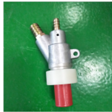
Fig. 2. Appearance of the nozzle for sandblasting
