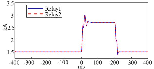
Fig. 8. Positive sequence currents at Relays 1 and 2 when the BC phase-to-phase short circuits occur at F2
