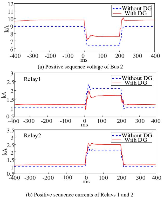
Fig. 3. Influence of the DG installation on the electrical parameters of the distribution network
