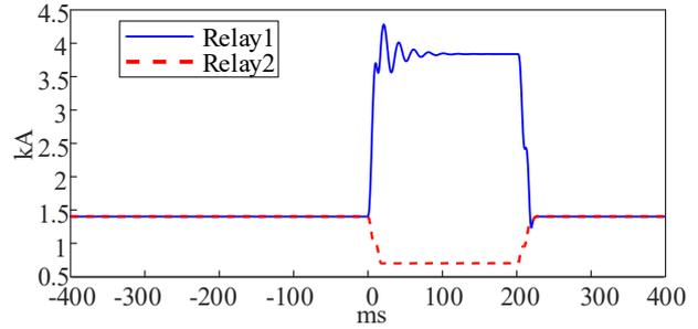
Fig. 7. Positive sequence currents at Relays 1 and 2 when the BC phase-to-phase short circuit occurs at F1
