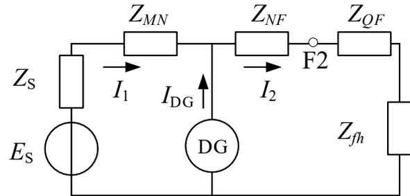
Fig. 2. Positive sequence fault network
