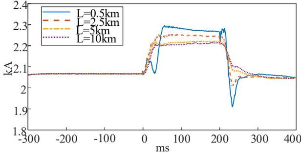
Fig. 4. Schematic of the DG output currents at different fault points
