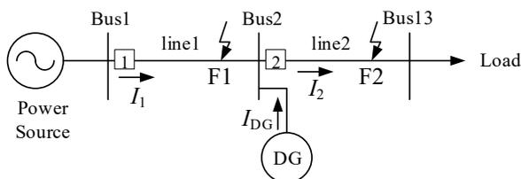
Fig. 1. Schematic of the distribution network with a DG
