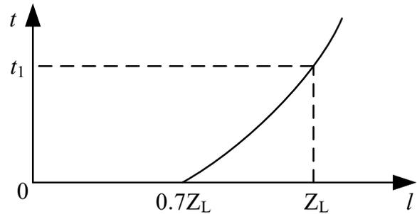
Fig. 5. Operating characteristics of adaptive inverse time current relay
