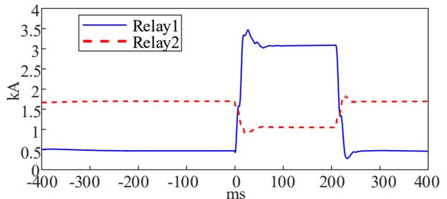
Fig. 9. Positive sequence currents at Relays 1 and 2 when the AB phase-to-phase short circuit occurs at F1
