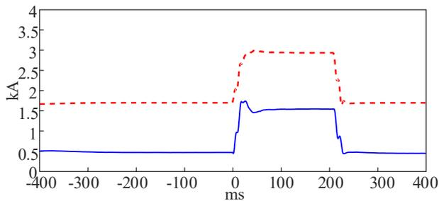
**Fig. 10.** Positive sequence currents at Relays 1 and 2 when the AB phase-to-phase short circuit occurs at F2
