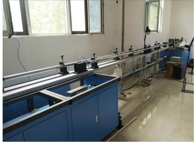
Fig. 3. Large-diameter split Hopkinson pressure bar system
