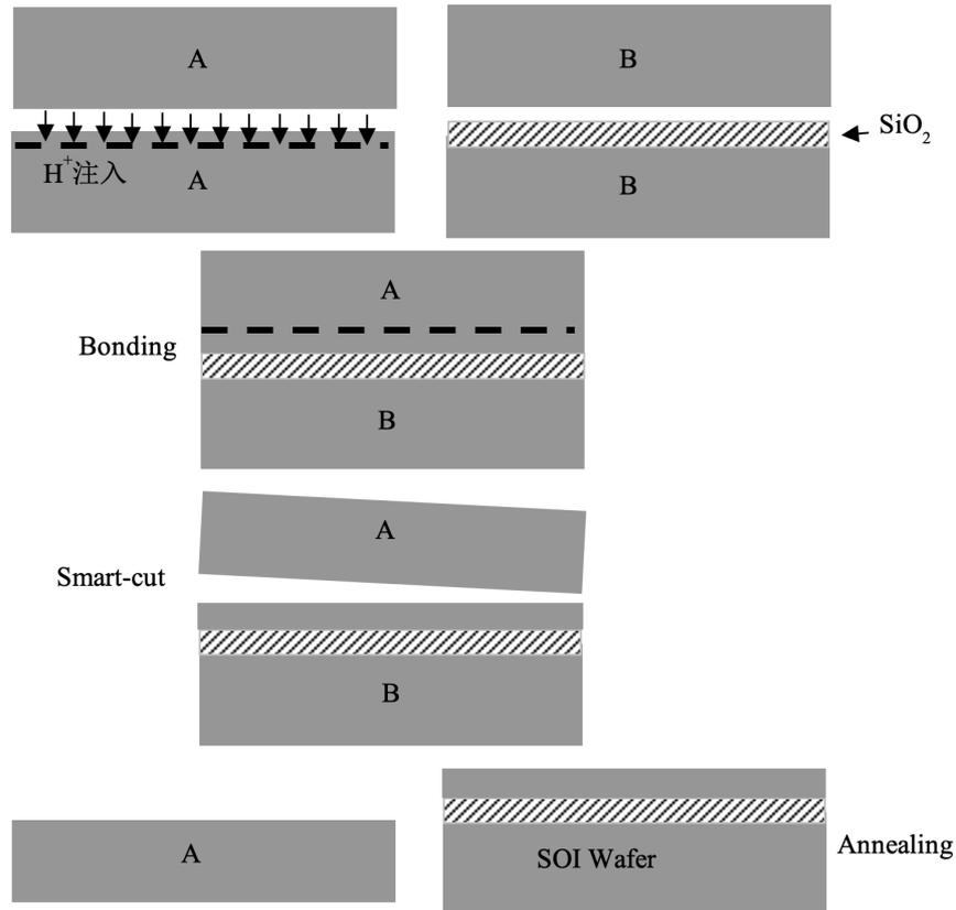
Fig. 2. Smart-cut process for SOI wafer
