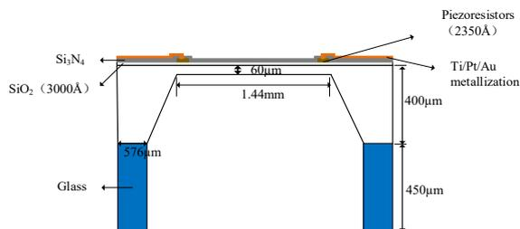
Fig. 3. Cross-sectional schematic describing the fabrication process of sensors
