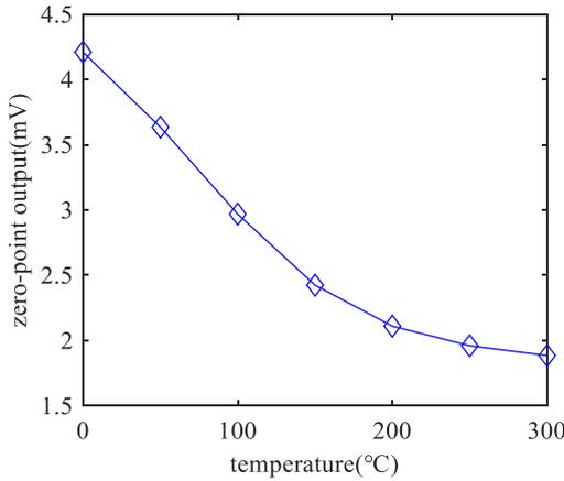
Fig. 9. Zero-point output vs temperature of the sensor
