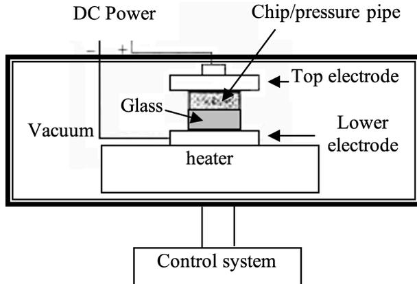
Fig. 4. Schematic of electrostatic bonding equipment
