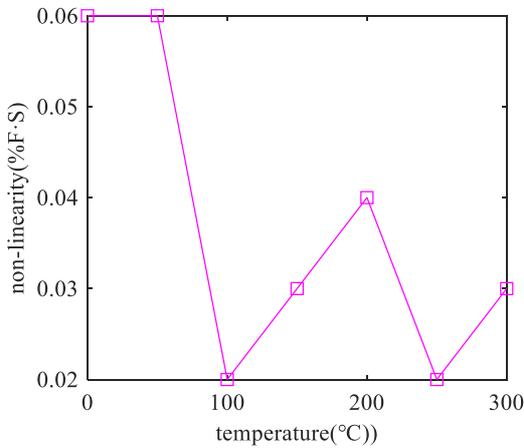
Fig. 10. Non-linearity vs temperature of the sensor
