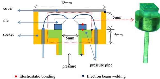
Fig. 5. All solid-state packaging structure based on silicon/glass/kovar alloy bonding
