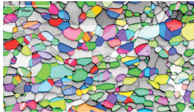
Fig. 3. Grain structure in a SAF 3207 HD umbilical tube Austenitic phase - Color grains are ferritic phase - grey grains. (Source: Guocai Chai et al, (2009), Sandvik Materials Technology)
