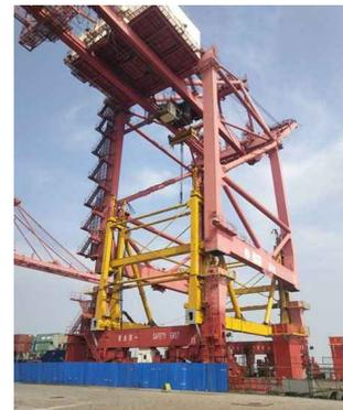
Fig. 9. Schematic of the hydraulic jacking device
