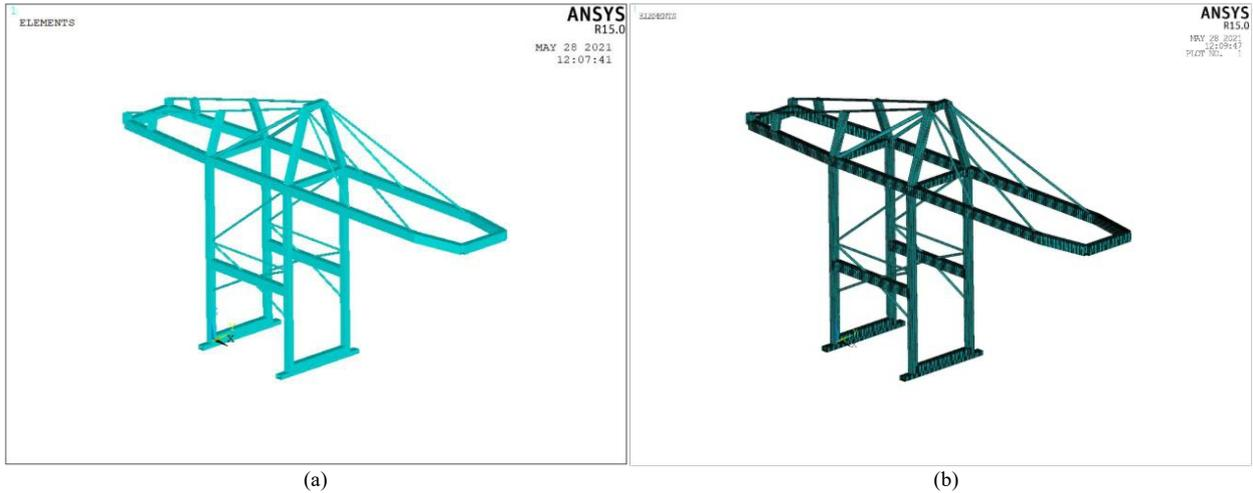
**Fig. 4.** Quay crane FEA model. (a) Metal structure geometry of the quay crane. (b) FEA model of the quay crane
