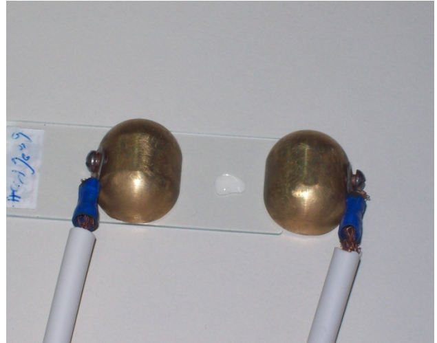
Fig. 1. Electrode arrangement with a water droplet on a borosilicate glass sample.
