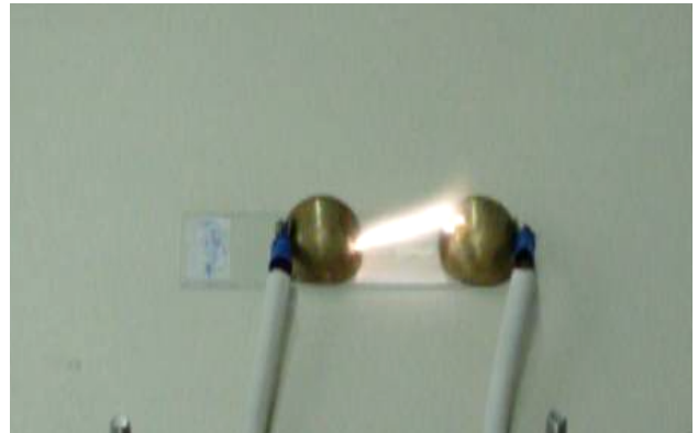
Fig. 2. Air flashover in a borosilicate glass sample.
