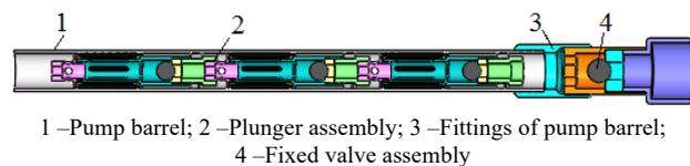
Fig. 1. Structural diagram of a three-stage soft plunger pump
