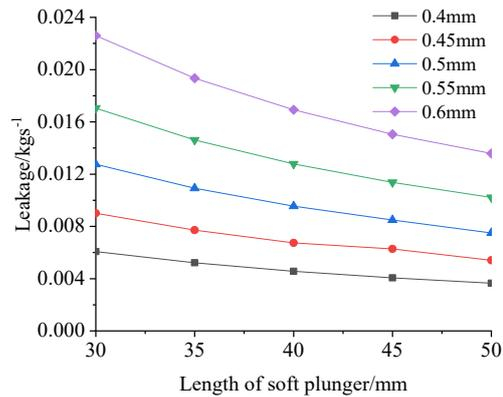
**Fig. 3.** Change curve of leakage with the length of the soft plunger
