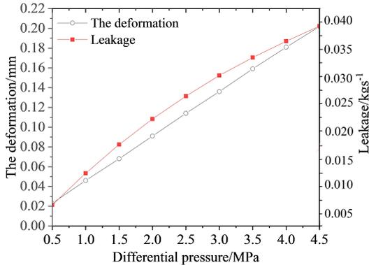
Fig. 4. Change curve of the leakage of the soft plunger and deformation with differential pressure
