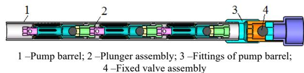
Fig. 1. Structural diagram of a three-stage soft plunger pump
