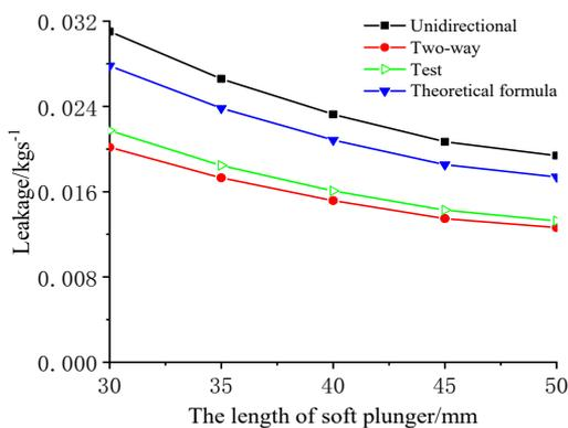
Fig. 5. Comparison of calculation methods under different length conditions
