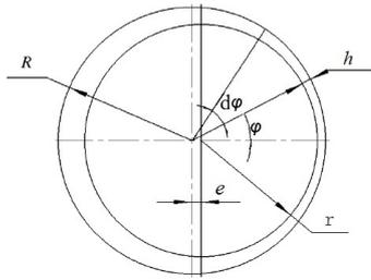
Fig. 2. Flow in an annular clearance
