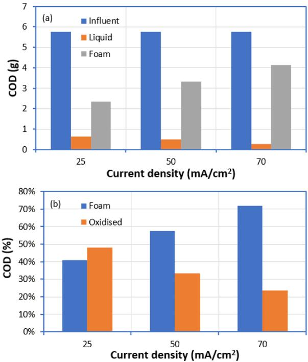
Fig. 3. (a) Mass balance of influent, effluent and foam COD, and (b) percentage of COD transfer to the foam and oxidized, by the applied electrooxidation process at different current densities after 4.5 h processing time.
