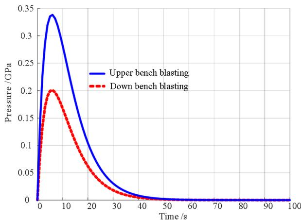
**Fig. 4** Time-history curves of explosive load for upper and lower benching blast
