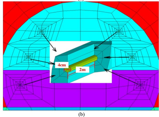
Fig. 3. The finite element model for blasting simulation in software ANSYS. (a) 3D numerical model of cross tunnels. (b) Zoom of the 3D simulation model and the arrangement of blasting holes
