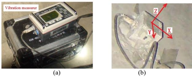
Fig. 1. The equipment for monitoring vibration. (a) TC-4850 for receiving electrical signals from sensors. (b) Installation of the TCS-B3 sensor
