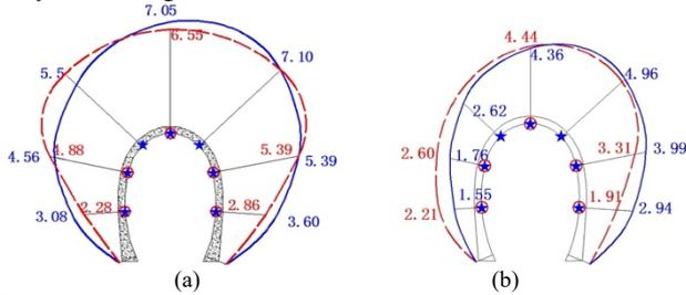
**Fig. 5** PPV distribution at the cross-section HDYK61+888 in the existing tunnel (a) PPV distribution was induced by the blasting at the upper bench in the new tunnel. (b) PPV distribution was induced by the blasting at the lower bench in the new tunnel.
