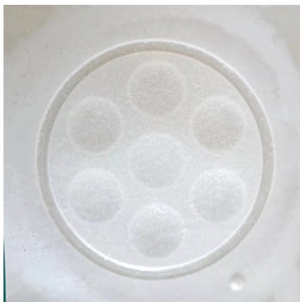
Fig. 13. Side subjected to water pressure
