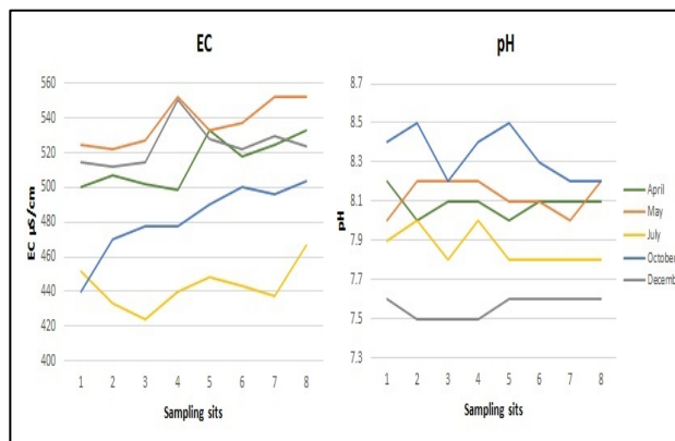
Fig.4. Graphs showing the variation of pH and Electrical Conductivity EC for the water samples within Tigris River in Mosul.
