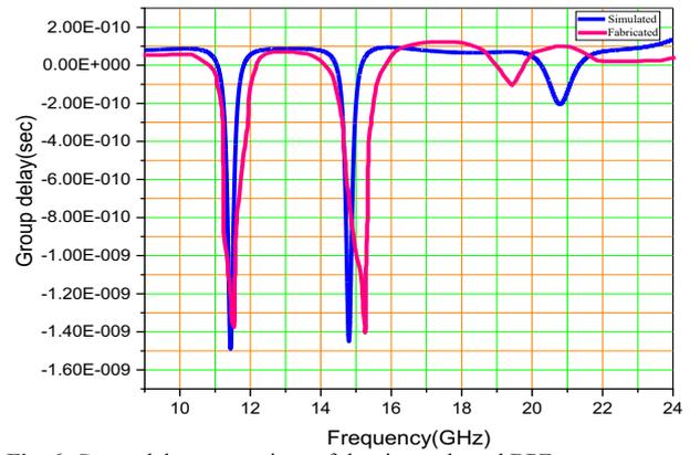
Fig. 6. Group delay comparison of the sigma shaped BPF.
