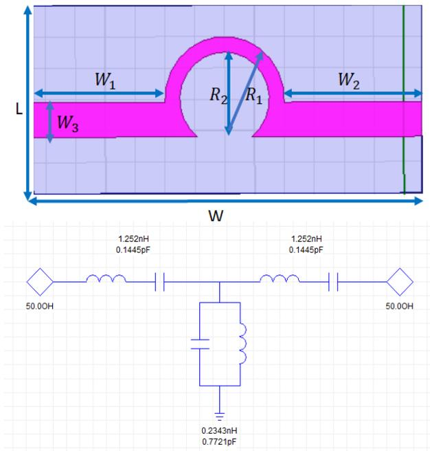
Fig. 1. Top view of the sigma shaped BPF and its circuit equivalent.
