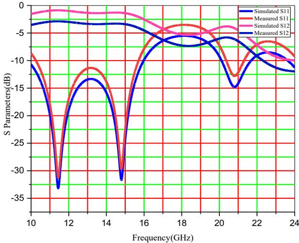
Fig. 5. S-parameters comparison of the sigma shaped BPF.
