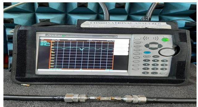
Fig. 3. Measuring the transmission Co-efficient by using Anritsu combinational analyser.
