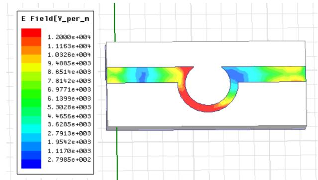
Fig. 7. Sigma shaped BPF's electric field distribution.
