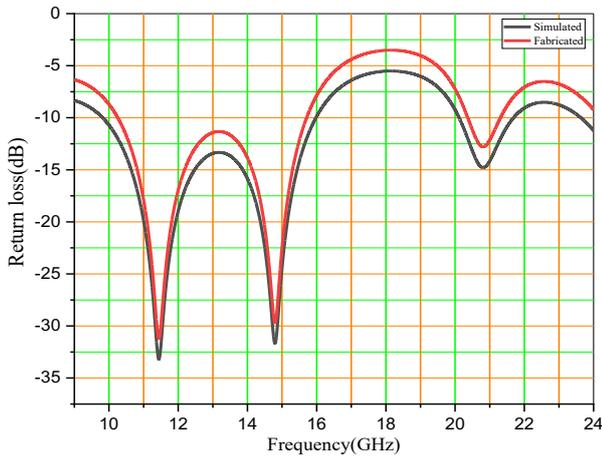
Fig. 4. Return loss comparison result of the proposed structure.
