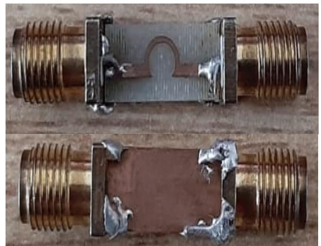
Fig. 2. Views of the fabricated sigma shaped BPF from top and bottom.
