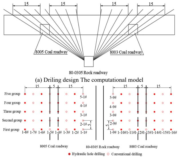
Fig. 4. Drill hole design and layout of final holes.
