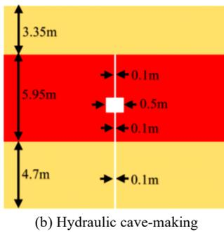
Fig. 2. Schematic diagram of numerical model and hydraulic cave-making.
