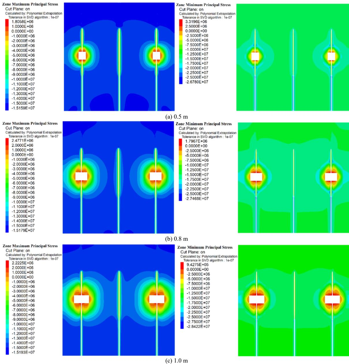
Fig. 6. Stress change of porous with different cave-making radiuses.
