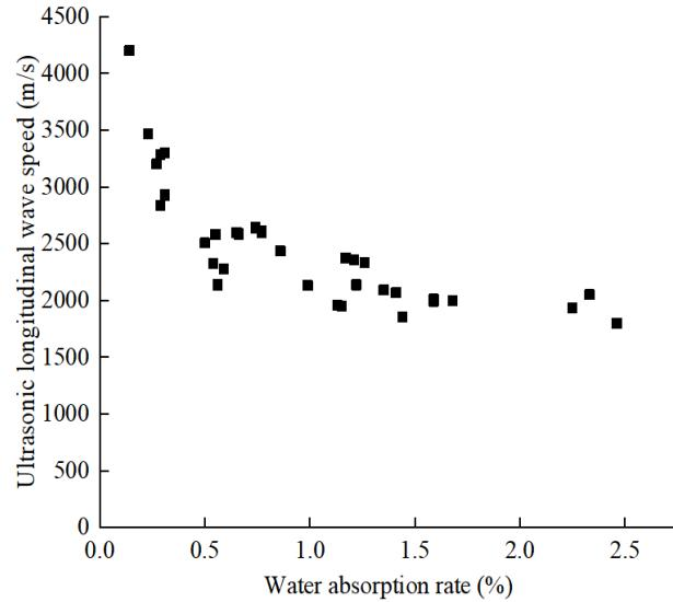
Fig. 7. Longitudinal wave velocity and water absorption rate of stone artifacts from Feilai Peak.
