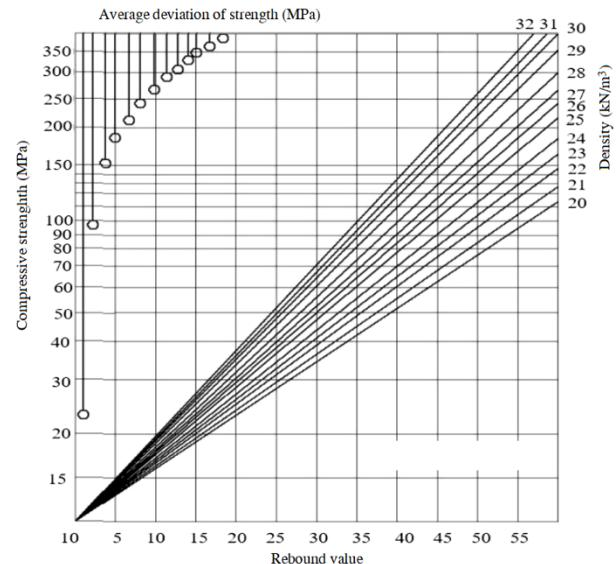
Fig. 1. Rock strength versus rebound value.
