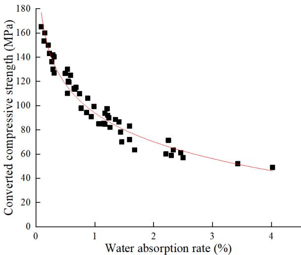
Fig. 6. The relationship between the strength of limestone surface layer and water absorption rate.
