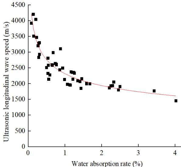
Fig. 9. Longitudinal wave velocity of limestone versus water absorption rate.
