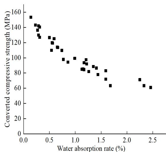
**Fig. 3.** Surface strength of cultural relics and water absorption rate relationship.
