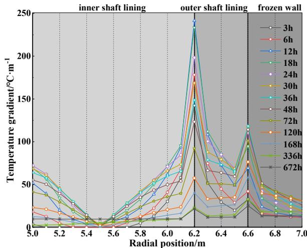
Fig. 10. Radial distribution of temperature gradient
