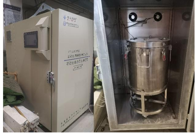
Fig. 4. BY-ATC/JR concrete adiabatic temperature rise tester
