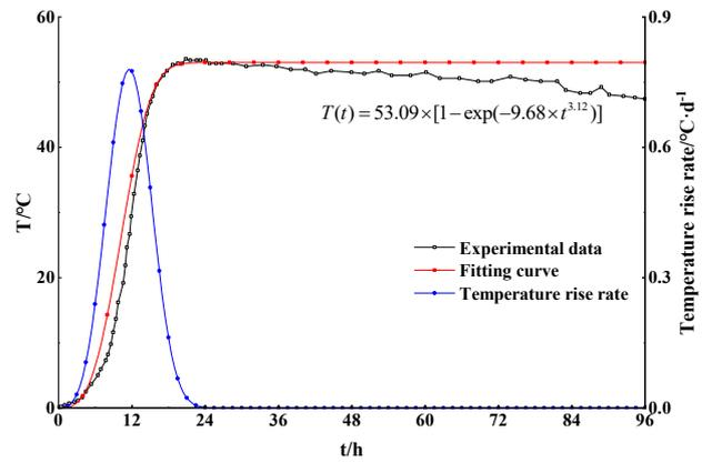
Fig. 5. Adiabatic temperature rise curve of C60 concrete
