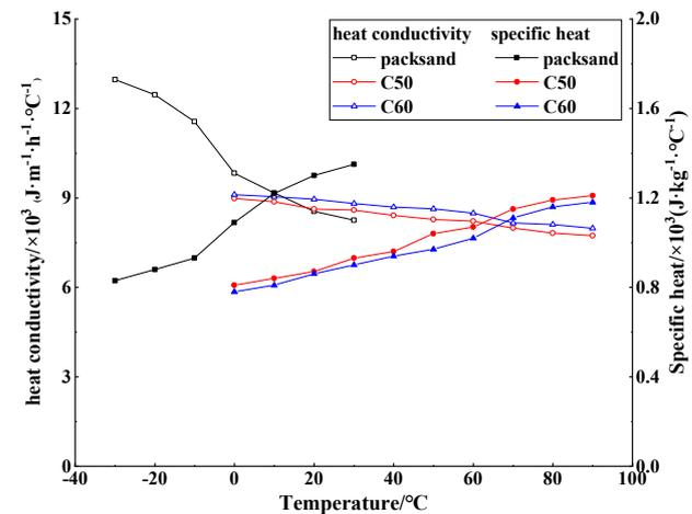
Fig. 6. Thermal conductivity and specific heat of specimens at different temperatures
