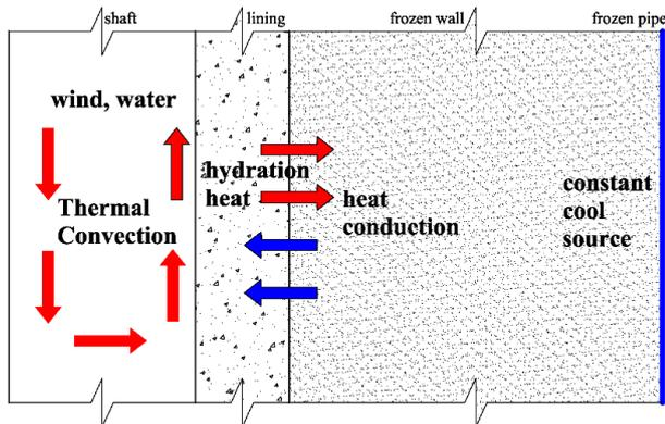
Fig. 2. Heat transfer mechanism for the temperature field of frozen shaft
