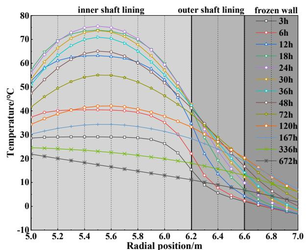
Fig. 9. Radial distribution of temperature
