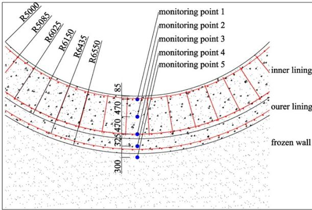
Fig. 1. Distribution of temperature sensors
