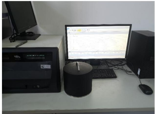
Fig. 3. Hot Disk TPS 2500S Thermal Constant Analyzer
