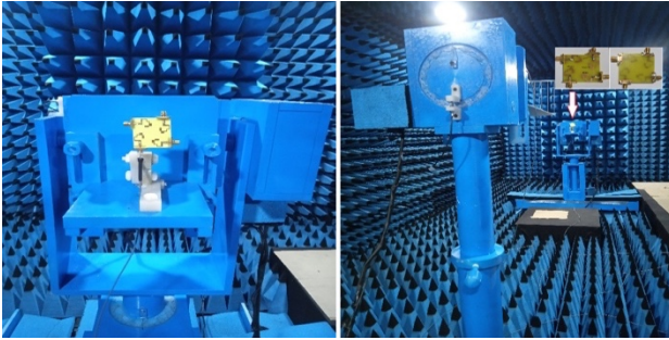
Fig. 9. Radiation Pattern Measurement in Anechoic Chamber
