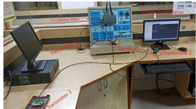
Fig. 13. Experimental Setup for Industrial Parameter Measurement
