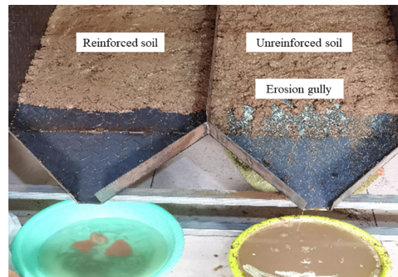
Fig. 12. Comparison of erosion forms of reinforced and unreinforced soil slopes
