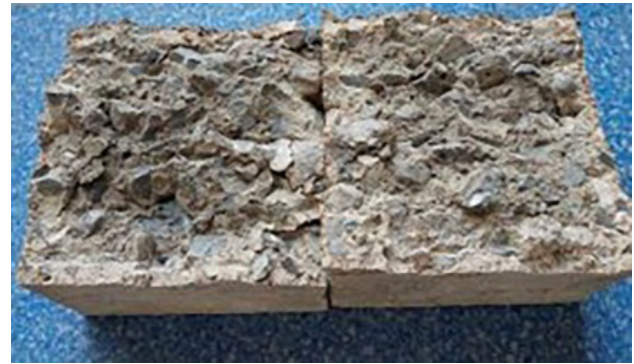
(e) \delta = 100\% \lambda = 0 \text{ kg}\cdot\text{m}^{-3} T = 600 \text{ }^\circ\text{C}
