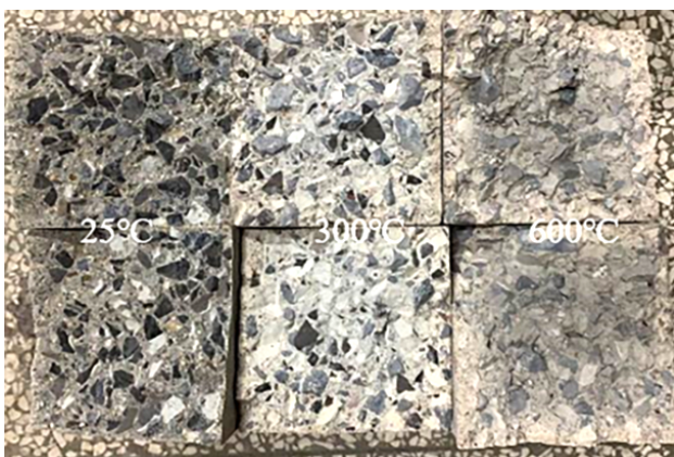
(b) \delta = 100\% \lambda = 4 \text{ kg}\cdot\text{m}^{-3} T = 25 \text{ }^\circ\text{C} - 600 \text{ }^\circ\text{C}
