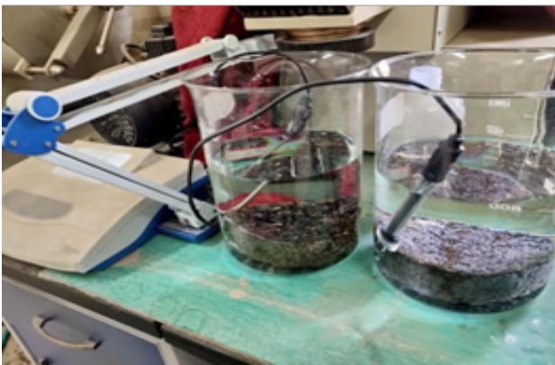
Fig. 2. Immersion conductivity test of salt-storage asphalt-mixture specimens
