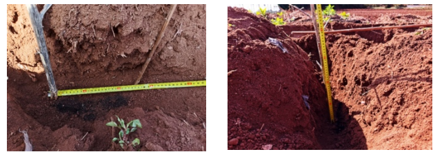
(a) Fertilizer width measurement (b) Fertilizer depth measurement Fig.22. Measurement of the effect of fertilizing operations
