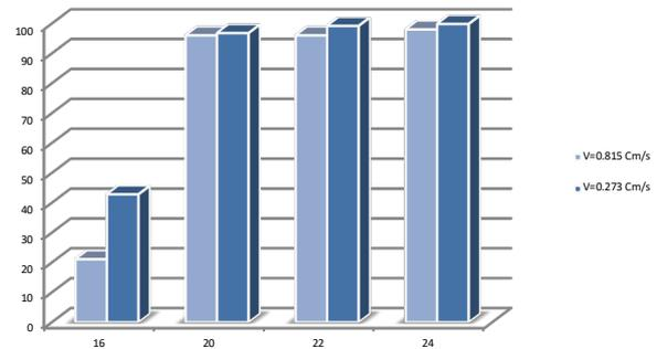
Fig. 8. Device cleaning efficiency for two displacement speeds as a function of voltage for L=30mm
