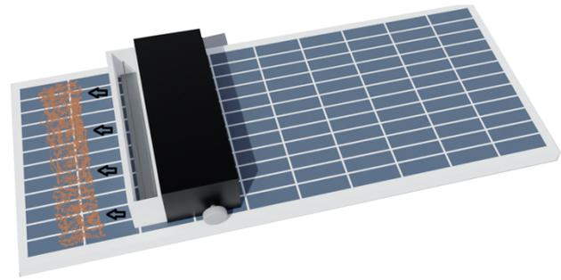
Fig. 2. Ionic wind actuator mounted on PV panel.
