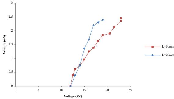
Fig. 6. Variation of wind velocity for different plate widths (L=20mm and 30mm).
