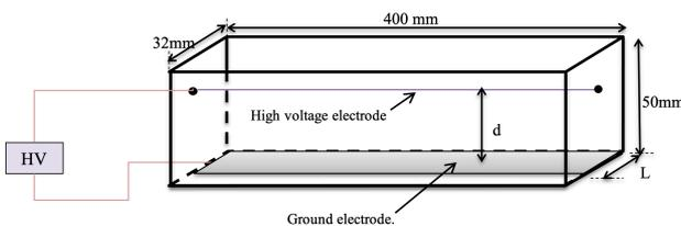
Fig. 1. Electrostatic cleaning system configuration.
