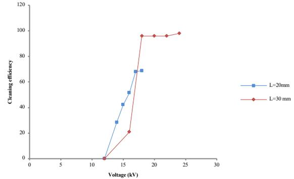
Fig. 7. Variation of cleaning efficiency as a function of voltage for different plate widths (L=20 mm and 30 mm).
