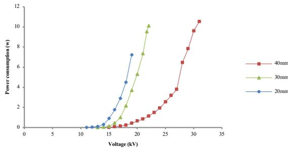
Fig. 3. Power consumption at different electrode gaps wire-plate (d=20, 30 and 40mm)
