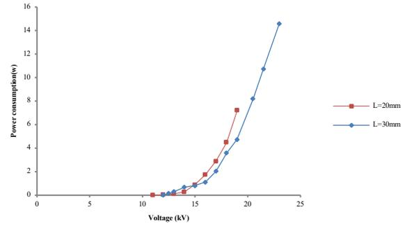
Fig. 4. Power consumption at different plate widths (L=20mm and 30mm).
