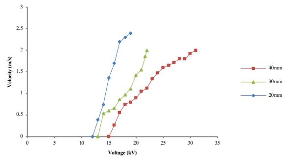
Fig. 5. Variation of wind velocity at different electrode gaps (d=20, 30 and 40mm)
