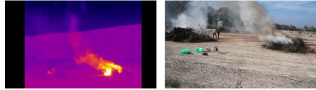
Fig. 6. Visual (right) and thermal (left) images of the time evolution of the two fires after 15 s (a, b), 30 s (c, d), 60 s (e, f), and 155 s (g, h), respectively, in all images, the right stack is quenched with water and the left stack with the BONPET-WATER mixture.
