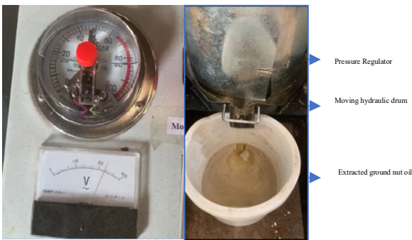
Fig. 4. Control unit and oil extraction through moving hydraulic drum
