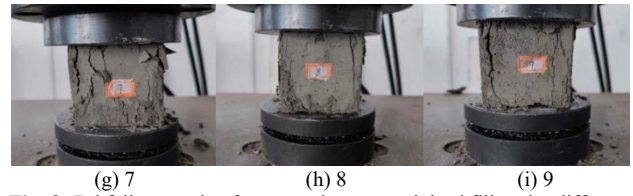
Fig. 8. 7 d failure mode of cemented waste rock backfill under different uniaxial compression tests.
