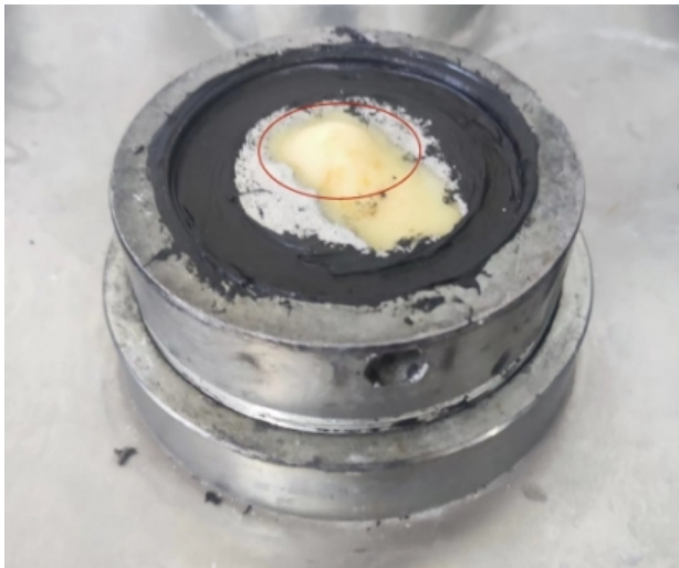
Fig. 18. Bulging of Grouting Materials
