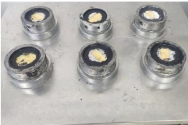
Fig. 9. Placement of the Impermeability Specimen
