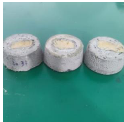
Fig. 7. Impermeability Specimen after Grouting
