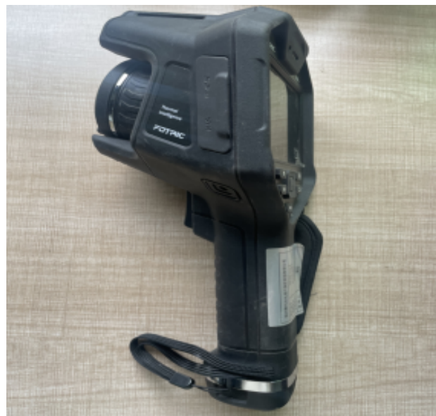
Fig. 2 FOTRIC 326Q handheld thermal imaging camera.
