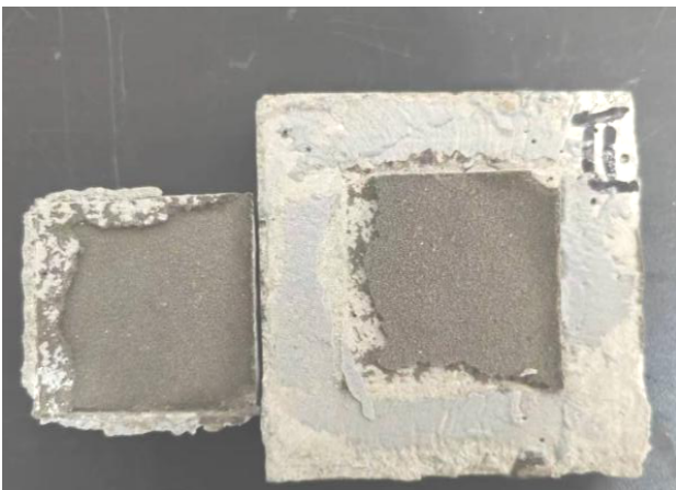
Fig. 20. Middle Failure in Bonding Test
