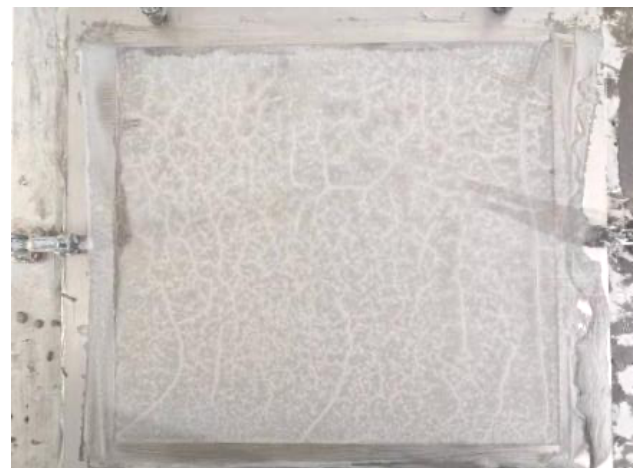
Fig. 10. Effect Picture of Film Formation with Rapid-Hardening Sulfate-aluminate cement
