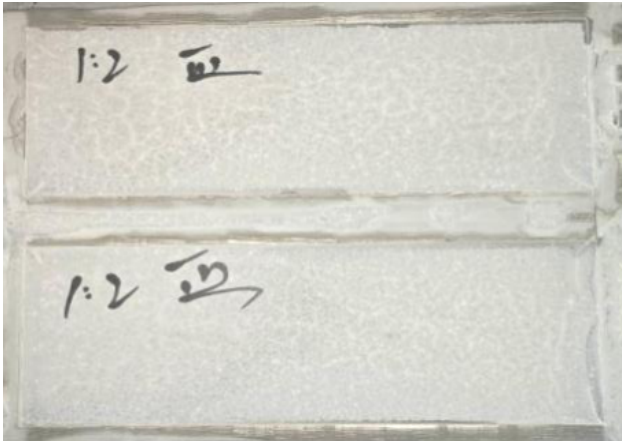
Fig. 11. Effect Picture of Film Formation with Rapid-Hardening Sulfate-aluminate cement
