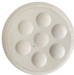
Fig. 16. Back Side Bulging of the Specimen
