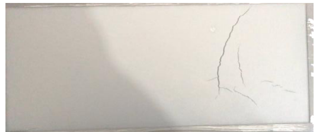
Fig. 9. Cracking of a Small Part of the Film
