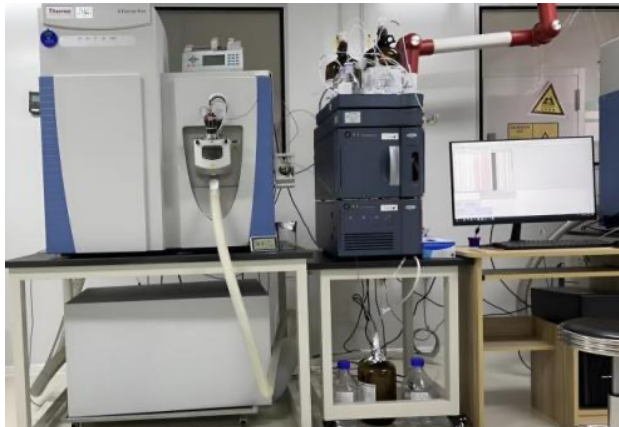
Fig. 2. Q Exactive Plus-combined quadrupole Orbitrap mass spectrometer
