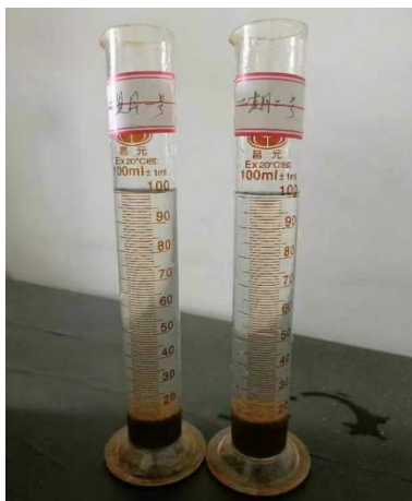
Fig. 2. Activated sludge at the end of the sewage aerobic biological treatment tank
