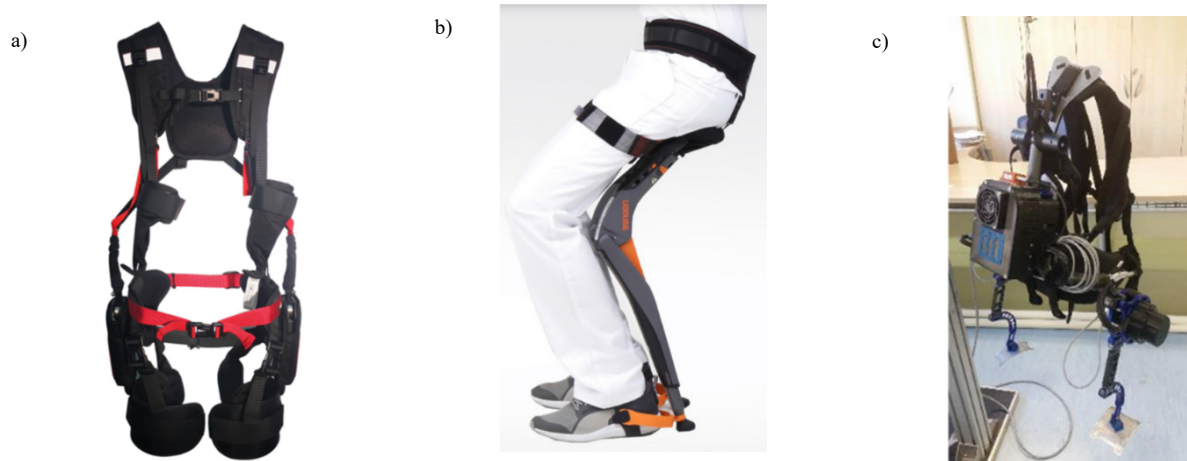
Figure 2. a) Upper passive exoskeleton IPAE [32], b) Lower passive exoskeleton Chairless Chair [12], c) Upper active exoskeleton [10].
