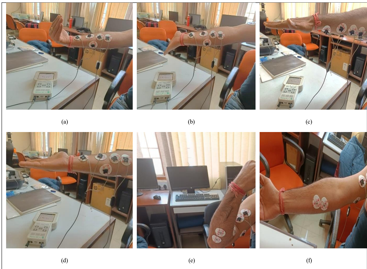
Fig. 1. Selected gestures. (a) WF: wrist flexion; (b) WE: wrist extension; (c) WP: wrist pronation; (d) WS: wrist supination; (e) EF: elbow flexion; (f) EE: elbow extension;
