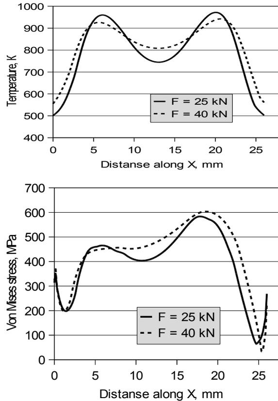
Fig. 3. The temperature and stresses distribution along the contact line for  $f = 50$  Hz,  $A = 1.5$  mm, (—)  $F_l = 25$  kN at the  $t = 0.72$  s, (- -)  $F_l = 40$  kN at the  $t = 0.62$  s
