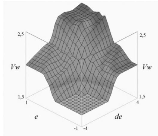
Fig. 5. Controller surface for designed FL controller
