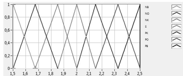
Fig. 4. Membership functions for travel speed
