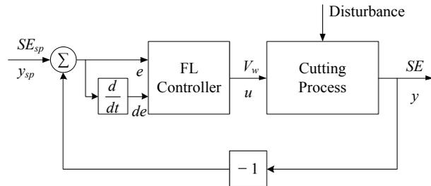
Fig. 3. Control loop with FL controller
