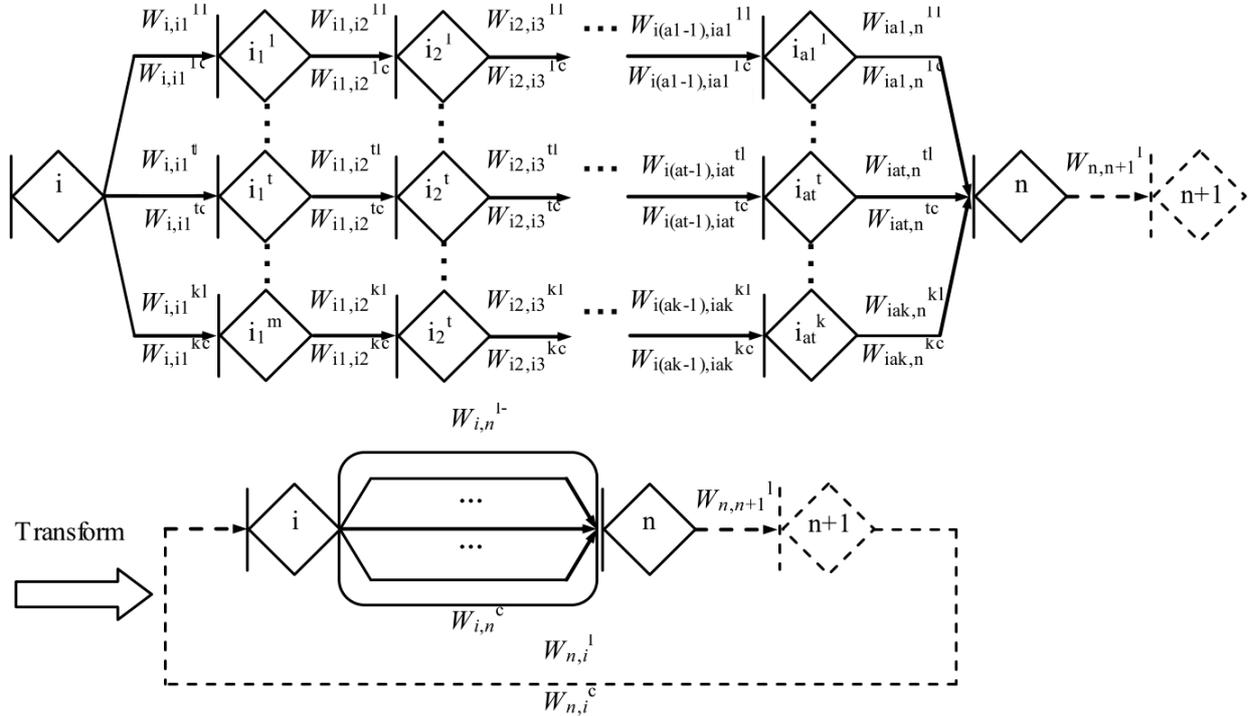
Fig. 5. Equivalent parameter calculation schematic diagram of parallel structure
