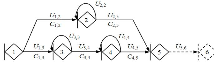
Fig. 3. The structural schematic diagram of quality gain-loss transmission GERT network
