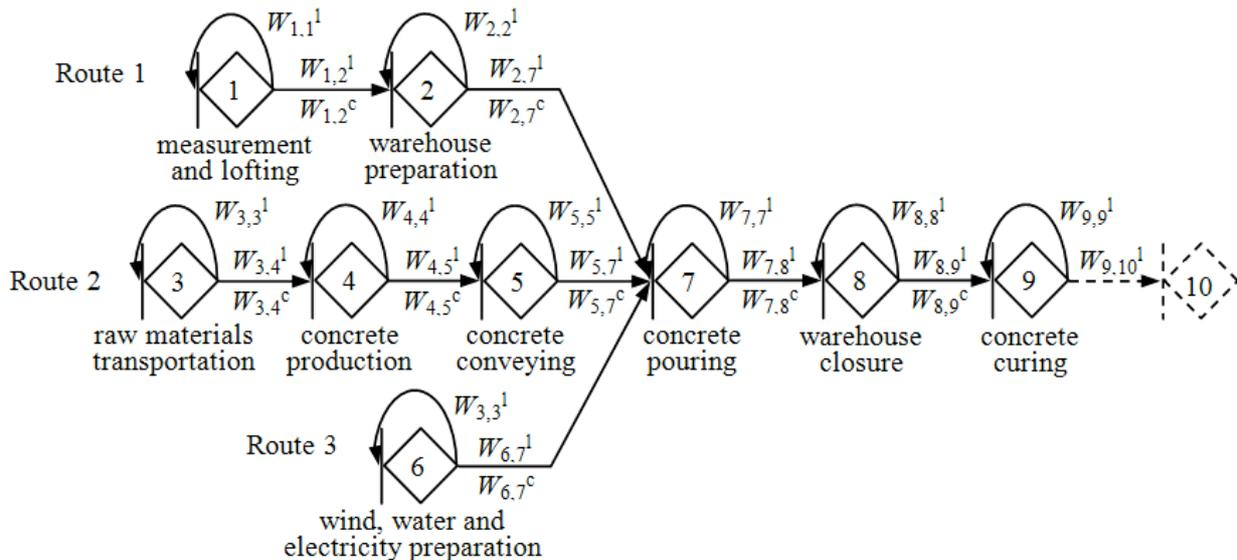
Fig. 7. Quality gain-loss transmission GERT network model of dam concrete construction in summer
