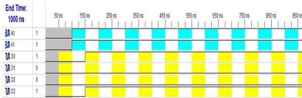
Fig.5.Simulated results of the reversible squaring circuit
