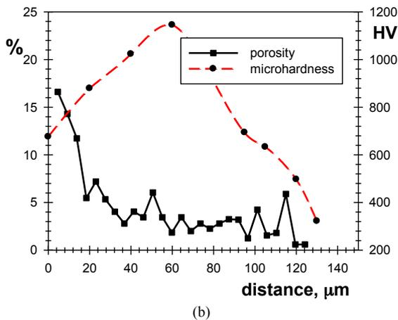
Fig. 4. Porosity and microhardness of the coatings along the sample surface: a) sample №1, b) sample №2
