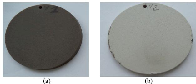
**Fig. 1.** Samples of the AK12D alloy after MAO: a) sample №1, b) sample №2
