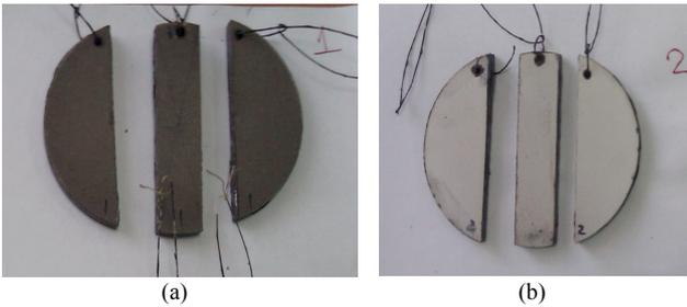
Fig. 3. Samples of the alloy AK12D after the corrosive tests: a) sample №1, b) sample №2
