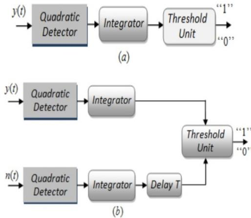
Fig. 5. Non-coherent receiver structures for DCC system.
