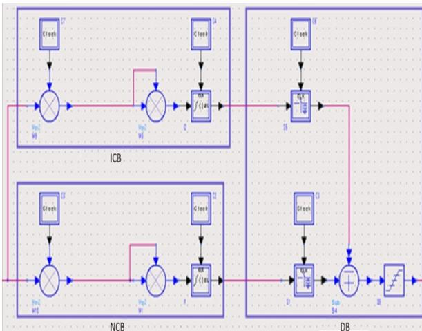
Fig. 10. ADS architecture of the AT-COOK receiver.
