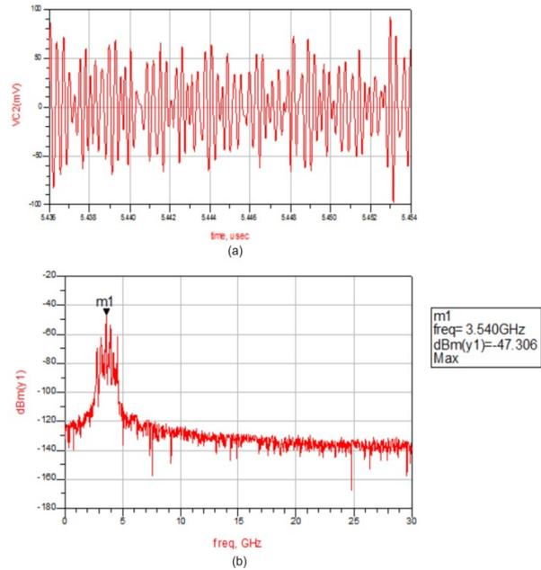
Fig. 4. ADS simulation results of the MCO signals after bandpass filtering: (a) The filtered signal  $V_{C2}$  and (b) The spectrum of the filtered signal  $V_{C2}$ .
