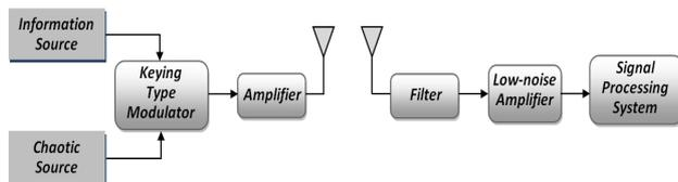
Fig. 1. Block diagram of the DCC system.
