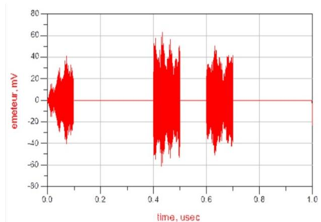
Fig. 8. CRP trains of UWB DCC COOK transmitter.
