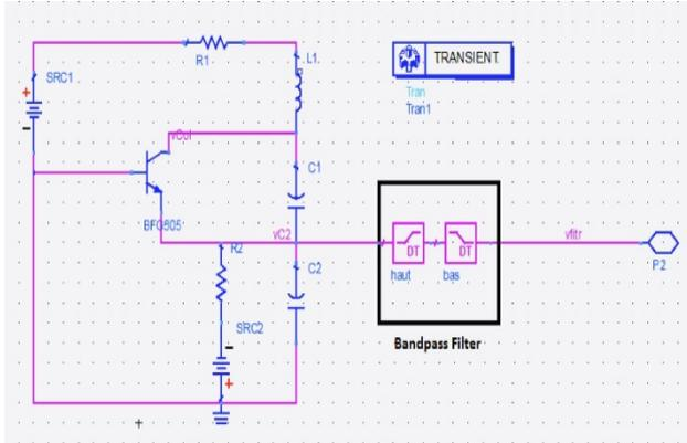
Fig. 2. ADS description of the MCO architecture.
