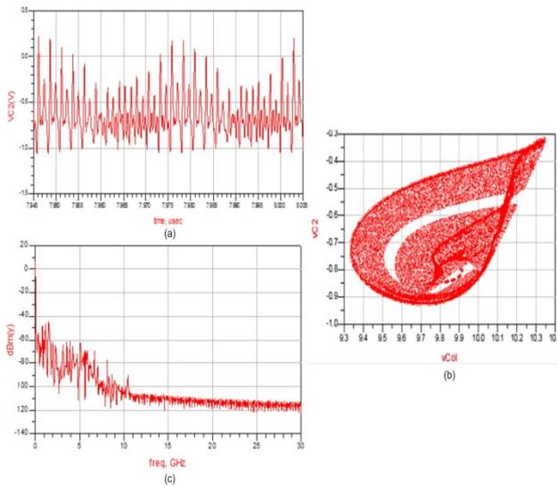
Fig. 3. ADS simulation results of the MCO signals before bandpass filtering: (a) Time-domain waveform of the voltage node  $V_{C2}$ , (b) The chaotic attractor in the  $V_{C2}$ - $V_{Col}$  plane and (c) The spectrum of the signal  $V_{C2}$ .
