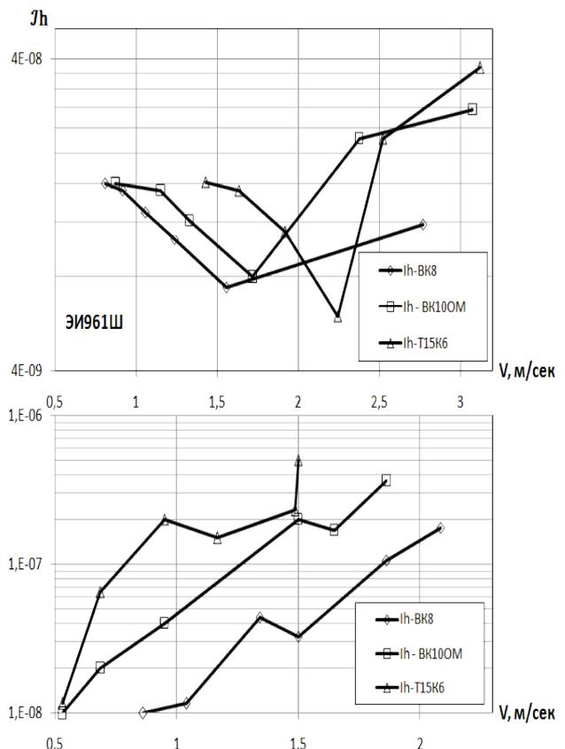
Fig. 1. Cutting speed effect on wear rate when turning Ni-based heat-resistant steel and Ti alloy by cutters made of various tool materials.
