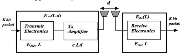
Fig. 4. Radio Energy Dissipation Model.
